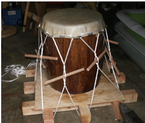
River Ridge Taiko on the "skinning stand", first stretch before attaching the head.
